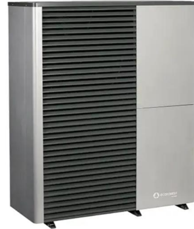
Typical 20kW floor standing air source heat pump. R290 refrigerant. Can be cascaded with up to 6 heat pumps operating in parallel.
