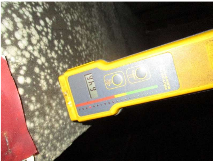
Photo 81 – Moisture content of timber 64%
