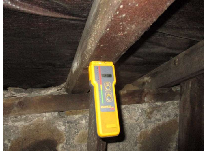
Photo 80 – Moisture content of timber 23%
