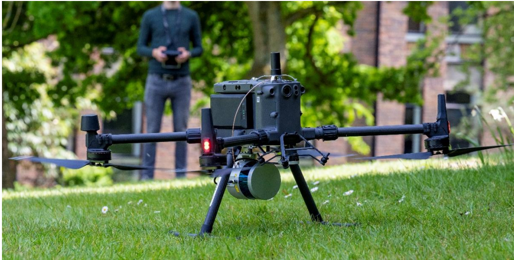
Figure 4: The DJI M300 RTK UAV with TopoLidar 100 sensor payload.
