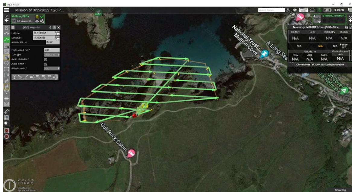
Figure 8: UGCS mission planning for a flight at Mullion Cove.
