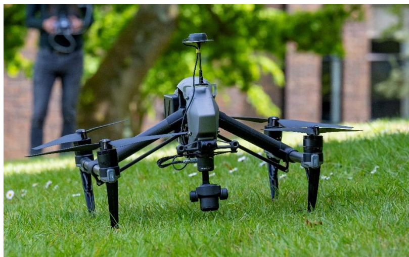
Figure 5: The DJI INSPIRE II UAV with modified X4S direct georeferenced camera payload.
