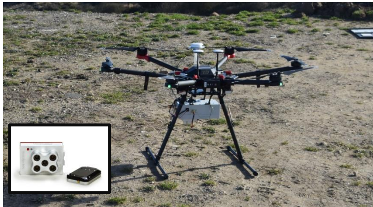
Figure 6: The DJI M600 Pro UAV with Micasense RedEdge MX (inset image) and Applanix APX15 INS payload.
