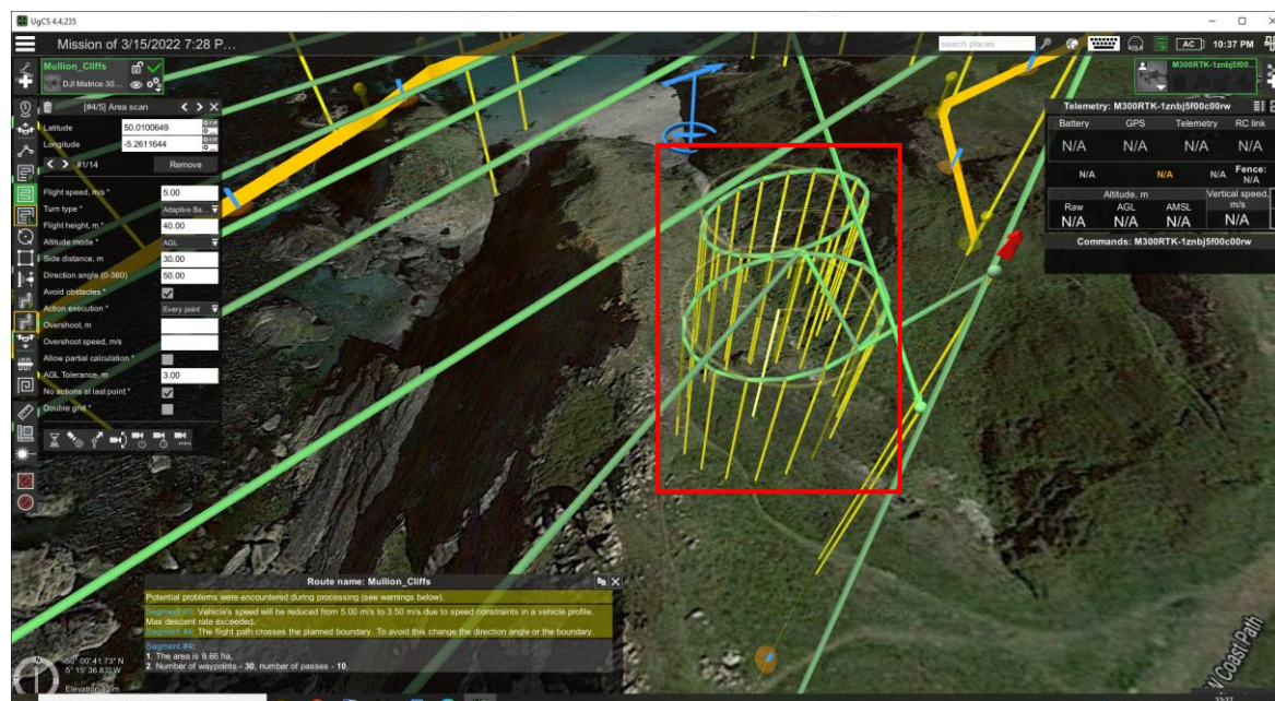
Figure 9: Detail of the inertial navigation system (INS) initialisation procedure planned in UGCS, consisting of a clockwise and anticlockwise circular flight path (highlighted in the red box).
