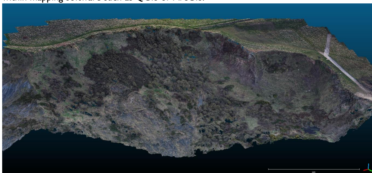
Figure 12: SfM output from Reighton, showing the ability of the software to build out accurate topography, but with a tendency to smooth features and lacking penetration through vegetation.
