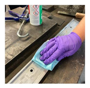
4) Apply a thin coating of LOCTITE SF 7515 using a lightly soaked lint-free cloth, or BONDERITE M-NT 1455-W pre-applied wipe. Leave to dry (5 – 10 minutes). This will convert the aluminium surface and prevent flash corrosion, protecting the surface and maximising adhesion. This treatment is active for ~48 hours and parts must be bonded within this time.
