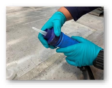
10) Attach the second nozzle to the TEROSON Multi-Press Spray Gun, over the top of the first nozzle.
