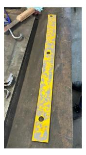
6) Mask/tape off the bolt holes. Applying masking tape to the edges of the sill plates and top face of the Treadmaster covering will also reduce post-application cleaning.
