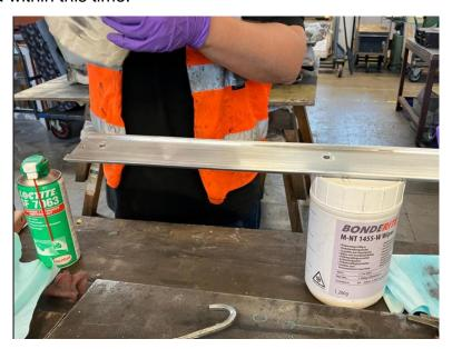
NOTE – THIS COATING MUST BE APPLIED TO RAW ALUMINIUM IMMEDIATELY AFTER ABRADING AND CLEANING FOR IT TO BE EFFECTIVE.
