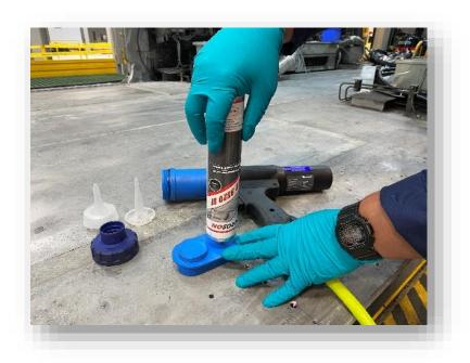
If using the TEROSON ET Multipress Pistol to dispense or spray the adhesive, steps 8 – 11 apply. If using a standard dispensing gun, fit the standard nozzle supplied with TEROSON MS 9320 SF to the cartridge and move to step 12.
