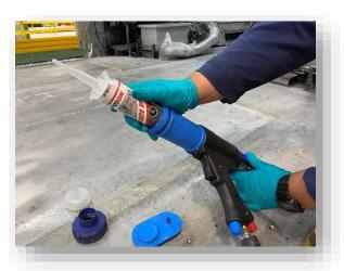
9) Attach the blue end cap over the cartridge and onto the TEROSON Multi-Press Spray gun – ensure that the blue cap is tightly secured, and a complete seal is formed by sufficiently compressing the O-ring on the dispense gun.
