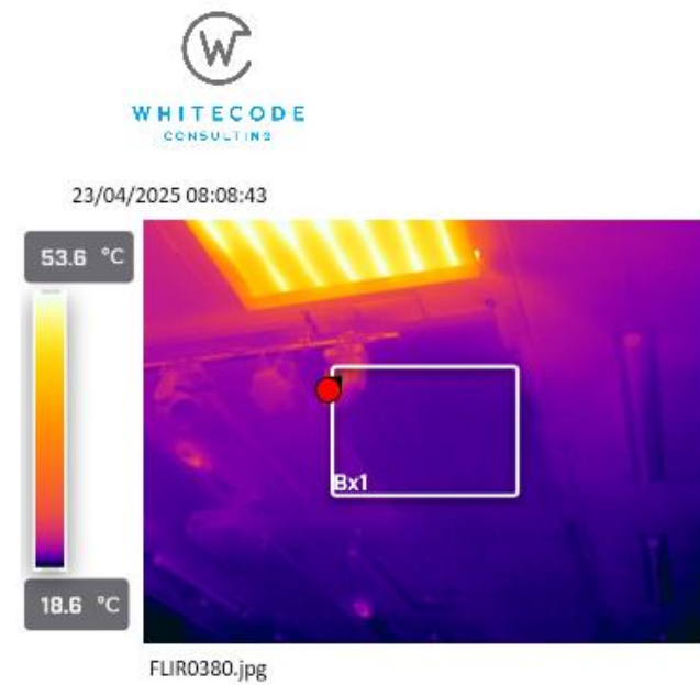
Image 4 – Only 25% of the radiant panels are operational
