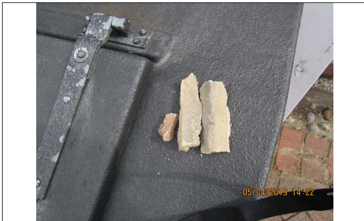
Photograph 35 Loose render collected from North and West elevations
