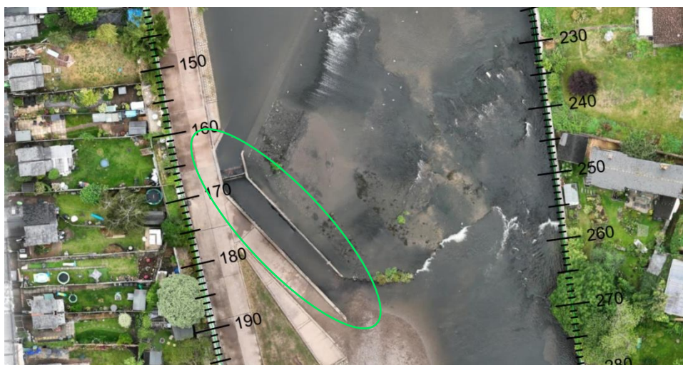
Figure 5 - Extract from chainage drawing 01 showing the stop-log structure and concrete wall downstream of it encircled in green.
